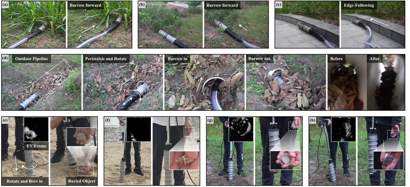
Fig. 22. Field experiments demonstrating SandWorm’s capabilities in real-world environments. (a) Moving forward in grass. (b) Moving forward in a bush. (c) Moving forward on a cement road. (d) Dredging in a blocked outdoor pipeline. (e)(f) Subsurface exploration experiment on the beach. (g)(h) Subsurface exploration experiment in composite garden soil. Full experimental footage is available in the supplementary video.
